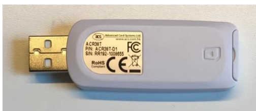
Illustration 13: "USB – chipcard writer"
