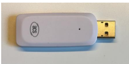
Illustration 12: "USB – chipcard writer"
